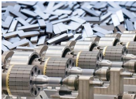
Fig. High performance Permanent magnets used for highly efficient electrical machines (Source: Siemens AG)
