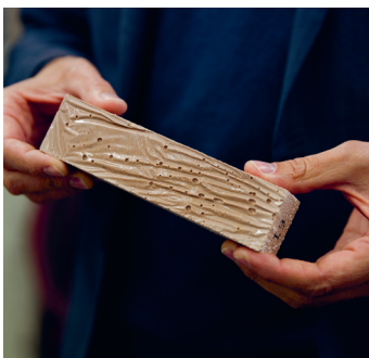
Geopolymer concrete flows into a form (top), cured test pieces (bottom).
