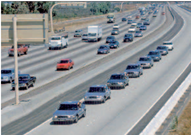
Abb. 4 Konvoi aus 8 automatisierten Pkw von California PATH/ University of Berkeley California, USA Automated 8 Car Platoon at California PATH/ University of Berkeley California, USA
