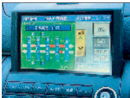
Photo 2 Examples of VICS traffic information displayed on the car navigation system
