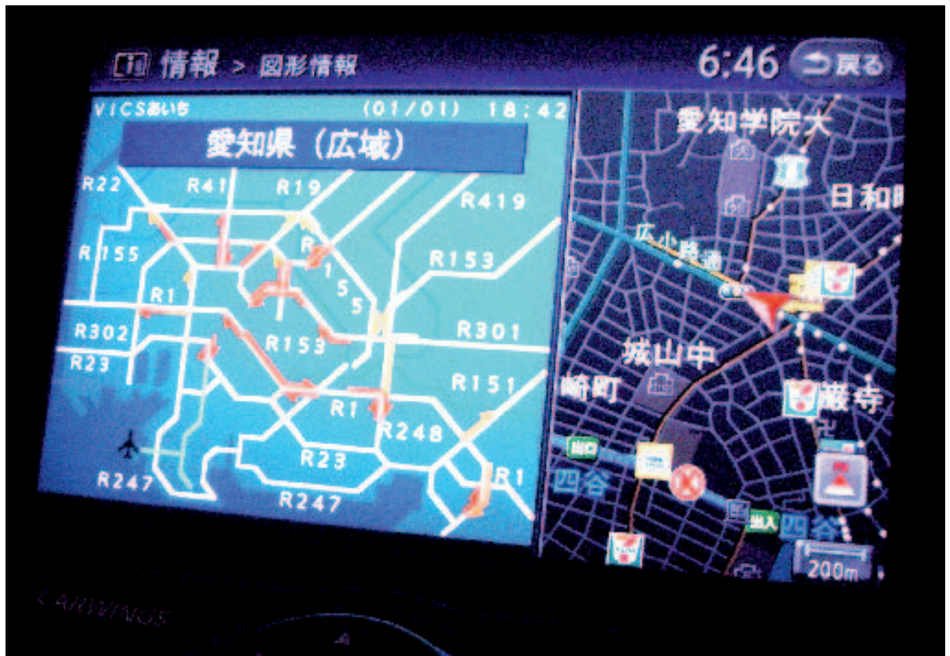
Photo 2 Examples of VICS traffic information displayed on the car navigation system
